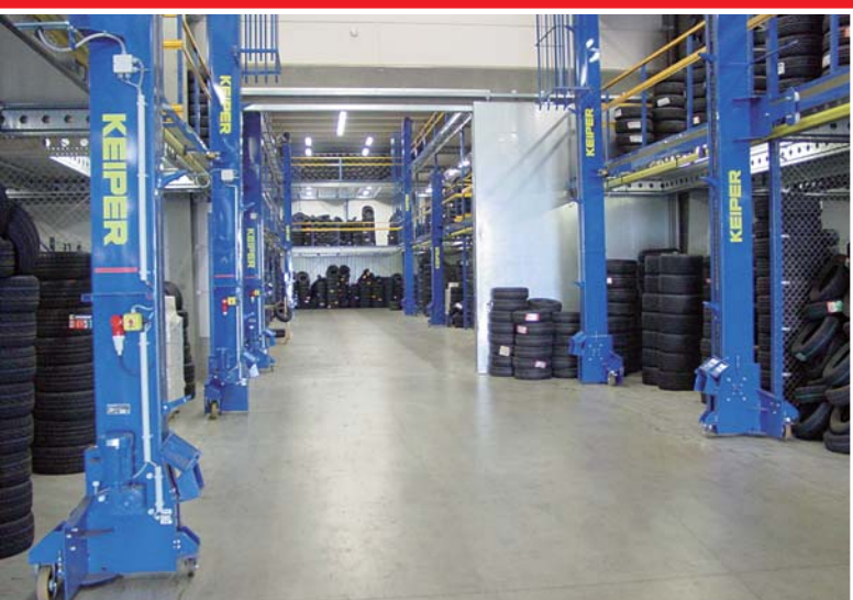
Special design of the tyre elevator for heavy truck tyres.
